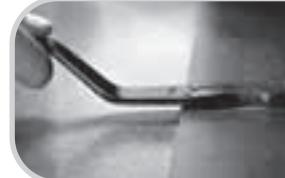
8a. For this, the actuating lever is moved into about middle position (primary air closed). If the flames now become weak, open the actuating lever slightly further (turn clockwise (+)).
