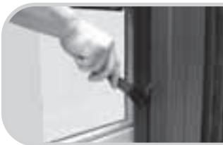
Move the 'cold hand' to the right-hand side of the door on the support/lock and turn it fully upwards.
