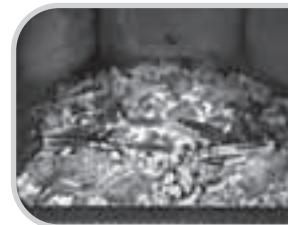
The end of the burning process is achieved when the wood has burned completely, and no smoldering or incomplete combustion can occur. Now the actuating lever can be closed (left position).
