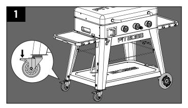
First, lock the two casters to immobolize the Cart. This will ensure the Cart does not shift or move once the Griddle is lifted.
