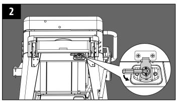
Unlock the latches on both sides of the Griddle. Push the latch lever downwards, then over to the opposite side to unlock the latch.
