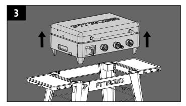
Using two people, lift the Griddle using the handles on each side. Lift until the feet of the Griddle have come completely out of the Cart.
